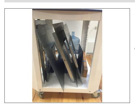
There are 3 different pairs of frames located below the vacuum former.
