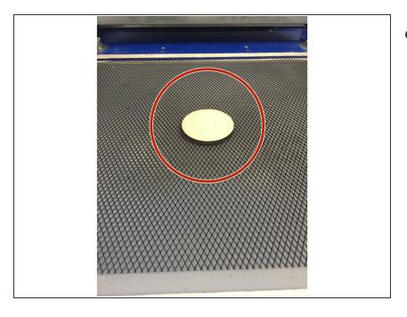
Place the object you want to mold onto the center of the bed.
