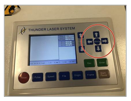
Move the engraver head to the top left corner using the right most arrows. Press the top arrow and the
