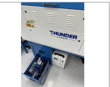
Underneath the Thunder Laser the last drawer contains the RotoBoss rotary chuck attachment.
