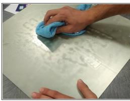
After you have removed your part, be sure to remove any remaining filament. Often a "skirt" or ring will be printed around the perimeter of your part. This skirt and all remaining filament should be removed from the print bed.
